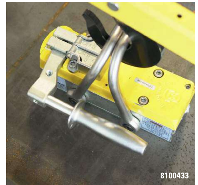
Lifting Manhole Cover with MagDolly
